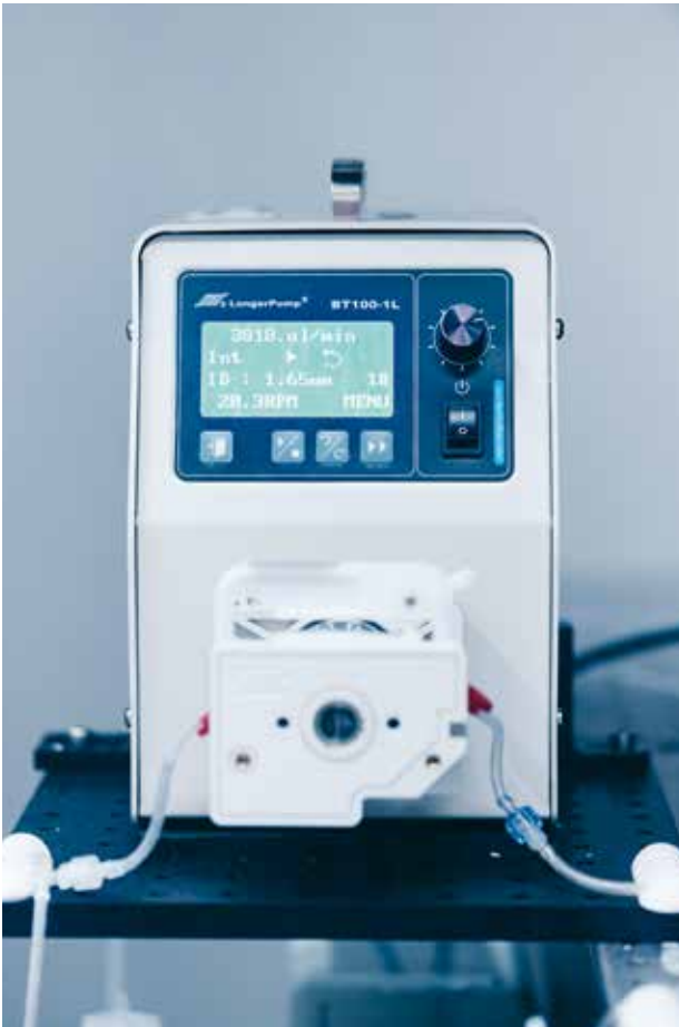
The flow rate, with the outflow managed by a pump, is at a constant 4 to 5 milliliters per minute.
